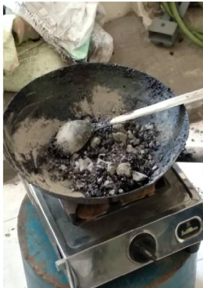
Fig 1: Mixing of Coated Aggregate and CRMB
