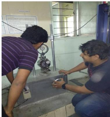
Fig 3 Marshall Stability test setup
