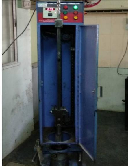
Fig 2 Automatic Marshall Compactor
